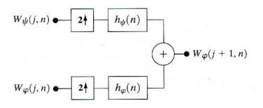
**FIGURE 7.18** The FWT<sup>-1</sup> synthesis filter bank.
