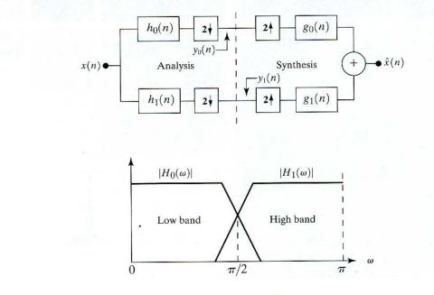
b FIGURE 7.4 (a) A two-band filter bank for onedimensional subband coding and decoding, and (b) its spectrum splitting properties.
