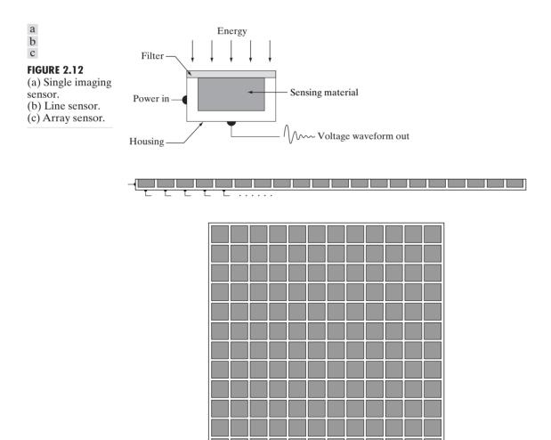
transformed into a voltage by the combination of input electrical power and sensor material that is responsive to the particular type of energy being detected. The output voltage waveform is the response of the sensor(s), and a digital quantity is obtained from each sensor by digitizing its response. In this section, we look at the principal modalities for image sensing and generation. Image digitizing is discussed in Section 2.4.
