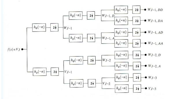
**FIGURE 7.30** The (a) filter bank and (b) spectrum splitting characteristics of a three-scale full wavelet packet analysis tree.
